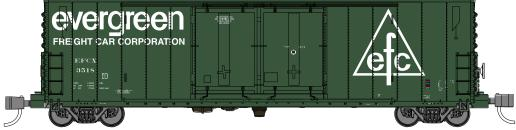
Evergreen Freight Car Corp. PC&F 50-ft 70 Ton Insulated Box Car, Double 8-ft Landis Plug Doors, Side Vents, (New BODY STYLE) 10 number series
